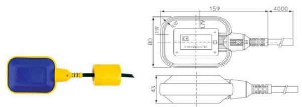
Item: WLY-2 Description: rectangle, blue ball Rated current: 10A Max. Temperature: 70°C Cable length: ≤20m Certification: CE CB SEMKO Widely used in sewage water, oil, acidic liquid, automatic fuel feed etc.
