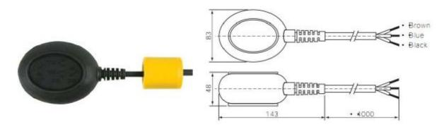
Item: WLY-5 Description: ellipse, black ball Rated current: 10A Max. temperature: 70°C Cable length: ≤20m Certification: CE CB SEMKO Widely used in sewage water, oil, acidic liquid, automatic fuel feed etc.
