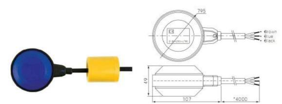
Item: WLY-4 Description: small circular, blue ball Rated current: 10A Max. temperature: 70°C Cable length: ≤20m Certification: CE CB SEMKO Widely used in sewage water, oil, acidic liquid, automatic fuel feed etc.
