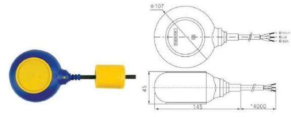
Item: WLY-3 Description: large circular, blue and yellow ball Rated current: 10A Max. Temperature: 70°C Cable length: ≤20m Certification: CE CB SEMKO Widely used in sewage water, oil, acidic liquid, automatic fuel feed etc.
